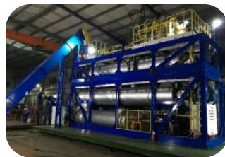
1.5 t/h Drill cuttings thermal desorption
