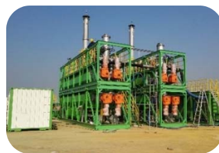
6 t/h Soil thermal desorption
