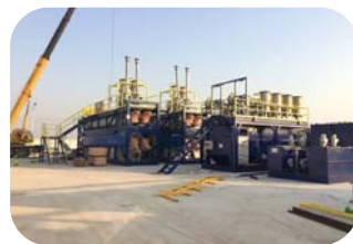
6 t/h double installation thermal desorption
